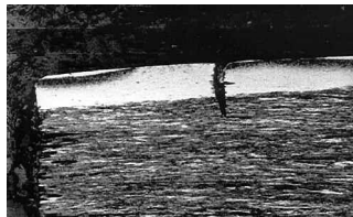
Wire section shown at high magnification: cracks begin to develop in the martensitic layer.
