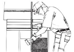
**5. SPOOL MULTIPLE LAYERS WITH SUFFICIENT TENSION.** It's very important to apply a tensioning load to the ropes during the rope breaking-in process. (If not, the lower layers may be loose enough that the upper layers become wedged into the lower layers under load, which can seriously damage the rope.) Improper tension can result in crushing and "pulling in" of the rope. The tensioning load should range from 2 to 3% of the rope's minimum breaking force.
