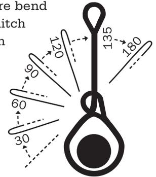
As always, if more than one sling is used and the legs are not vertical, a further reduction in rated capacity must be made for the sling angle.
