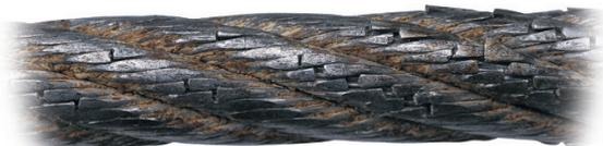
Shown here is a wire rope that has been subjected to repeated bending over sheaves under normal loads. This results in **fatigue breaks** in individual wires – these breaks are square and usually in the crown of the strands.
