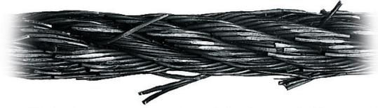
This is an example of **fatigue failure** of a wire rope subjected to heavy loads over small sheaves. The breaks in the valleys of the strands are caused by "strand nicking." There may be crown breaks, too.
