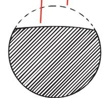
**CROSS-SECTION OF A PEENED WIRE**
