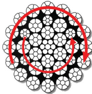
In standard 6- and 8-strand ropes, the torques produced by the outer strands and the IWRC are in the same direction and add together. In rotation-resistant ropes, the lay of the outer strands is in the opposite direction to the lay of the inner strands, thus the torques produced are in opposite directions and the torques subtract from each other.
